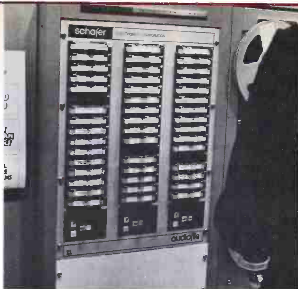
Another new item at NAB was the Schafer Audiofile. The drive system and heads move up and down while the cart remains fixed. Previous systems used a common drive system.
