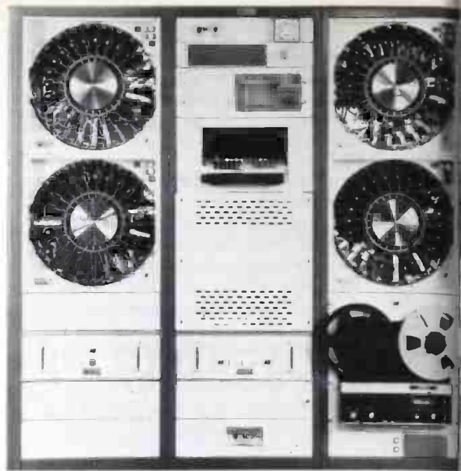
Automation system with digital control, the SMC DP-1. Alternate configurations might use more reel-to-reel playbacks.
